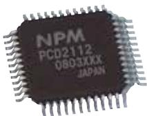
The first of its kind, this miniature package (mold measuring only 7x7mm) adopts a four-wire serial bus that enables downsizing of the board. It can output two-phase stepping motor excitation sequence and is equipped with a servomotor interface. The PCD2112 can control both stepper motors and servomotors.
